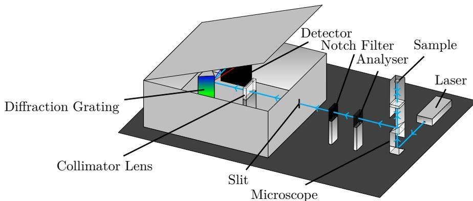
Figure 7: A schematic representation of the experimental setup used
